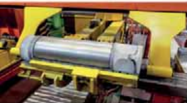
Jilin Liyuan, China: 45 MN Direct-Indirect-Tube Extrusion Press
