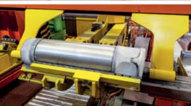
Jilin Liyuan, China: 45 MN Direct-Indirect-Tube Extrusion Press
