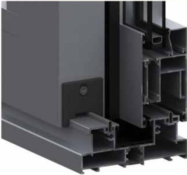
KSL-128 is thermal & high insulated lift and slide system. The sash weight can be until 250-300 kg and sash height can be until 3 meters. There is epdm gaskets between frame and sash and this makes the system high insulated. All European norm mechanisms can be use at the system.
