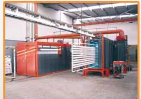
ELECTROSTATIC POWDER COATING EQUIPMENT
